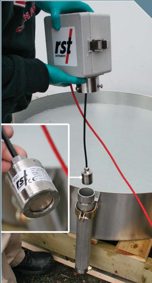
Close-up of the 4 - 20 mA transducer.
