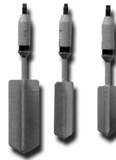
Vanes with slip coupling
