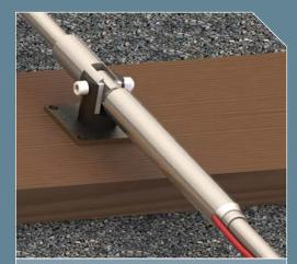
The Track Monitoring System is intended for monitoring settlement and twist of railroad tracks which may be affected by nearby construction activity, such as tunnelling or adjacent excavation, or which are located near hazardous zones such as potential washout or landslide areas.
